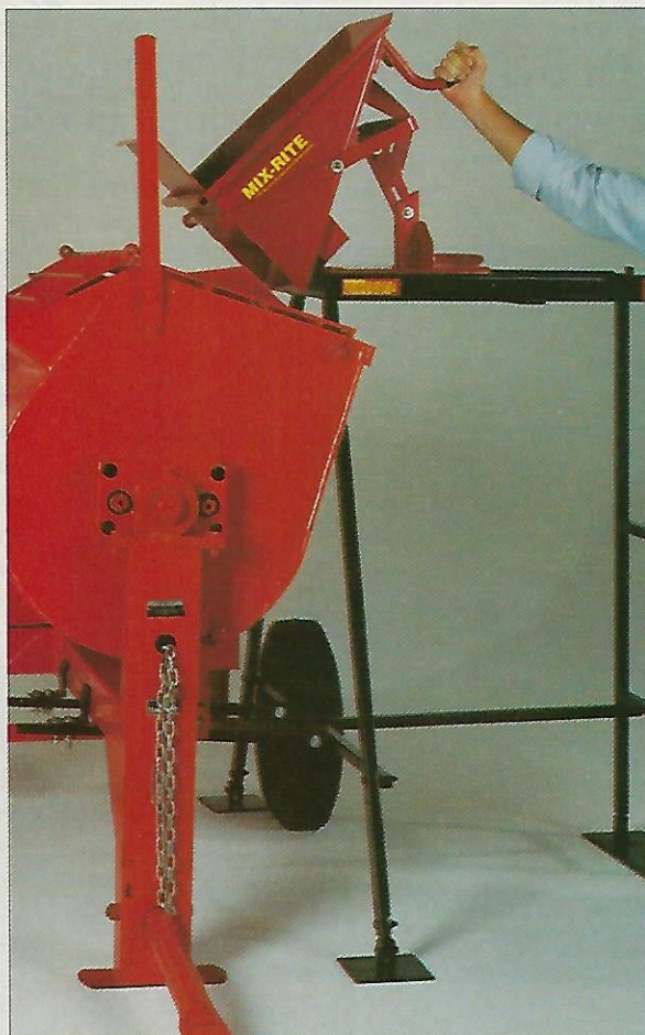
After loading the hopper with sand and pushing it forward to the end of the rails, operator pushes up on the handle—automatically opening the door at the wide end of the hopper and releasing 1 cubic foot of sand into the mixer.
